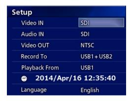
Move the cursor to the item to be set, and press the ENTER button to enable the item to be changed.
